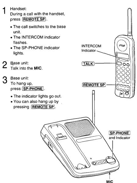
When using (REDIAL), dialing a stored number (p. 19), etc., press (REMOTE SP) after dialing is completed.
